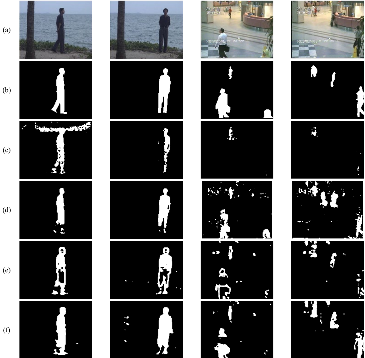
Figure 7: Foreground object detection for (a) two frames from the Watersurface video sequence (left) and from the Airport video sequence (right) together with their (b) ground-truth results. Object detection was performed using (c) MoG [23], (d) codebook model [12], (e) block-based eigenbackgrounds [17], and (f) the proposed method. The proposed method shows improved results compared to other techniques.
