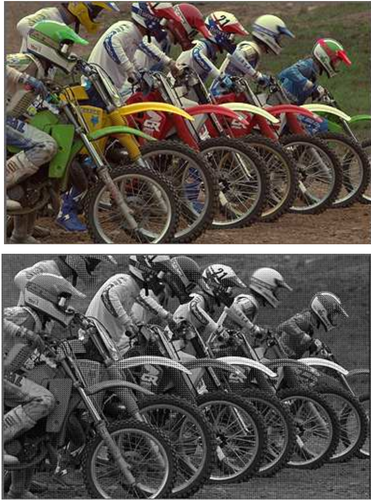
Figure 15: Top: The original RGB image. Bottom: A mosaic image which was sampled from the original image using the Bayer CFA.
