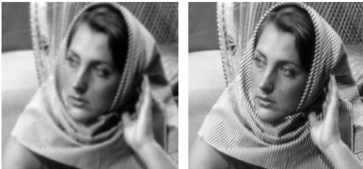
Fig. 17. Left: Blurred Barbara after applying a 5-tap Gaussian blur. Right: Sharpened Barbara using LUTs that were trained on blurred Lena using 8 \times 8 over-complete DCT.
