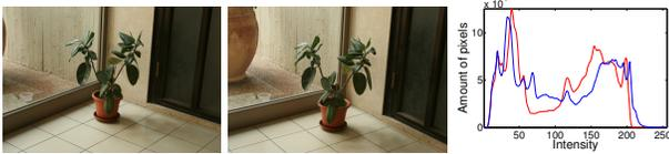
Figure 1. A degenerate case of two images taken from different viewpoints under the same illumination with the same camera and same photometric parameters. Note that the identity color mapping is correct although the histograms of the two images are different (right plot).
