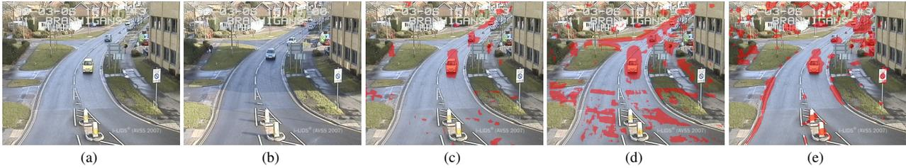
Figure 8. (a) and (b) show two images from different frames of a time-lapse video. Areas detected as different are marked in red. (c) shows change detection using our method; (d) shows change detection using normalized gray-scale correlation; and (e) shows change detection using image chrominance comparison. *Images taken from i-Lids vehicle detection challenge.*
